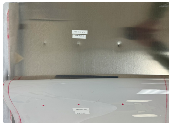
1" Hail Damage at 45 MPH Metal Thickness: .020"
