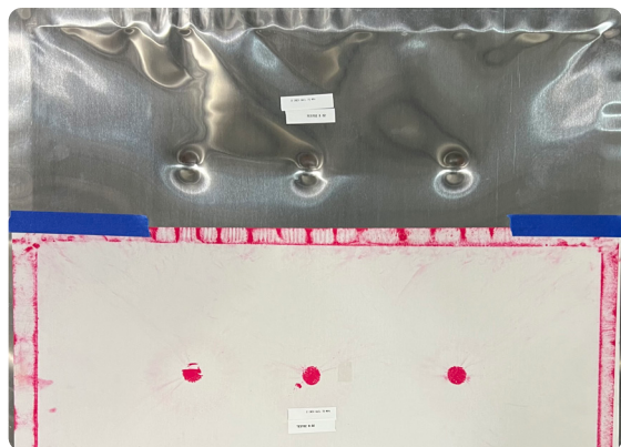
2" Hail Damage at 72 MPH Metal Thickness: .020"
