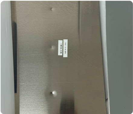
1" Hail at 45 MPH Metal Thickness: .020"
