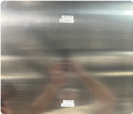
1" Hail at 45 MPH Metal Thickness: .020"
