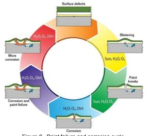
Figure 2. Paint failure and corrosion cycle.
